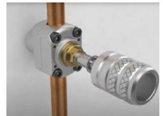
**Step 4:** Remove drill collar by hand and discard.
