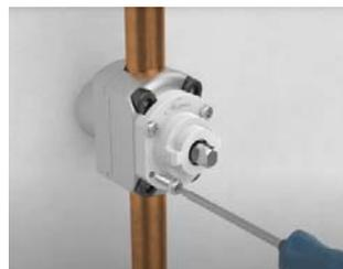
**Step 7:** Fit white plastic valve cap over spindle. **Gently push cap down to contact point with upper body**. Drive cap screws with phillips screwdriver.
