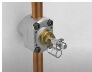
**Step 6:** Remove the split poly tube from spindle. **Do not remove the circlip.**
