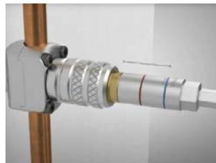
**Step 3:** Using drill on **low speed, high-torque setting**, drive cutter plug into valve. Use color reference lines as stop point. **Maintain consistent pressure** through **\*3 stages\*** as copper pipe is cut and seated.
