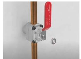
**Step 8:** Fit handle over spindle and use half nut to secure in place. Turn handle 90° to close valve. Valve action should be smooth with positive shutoff.
